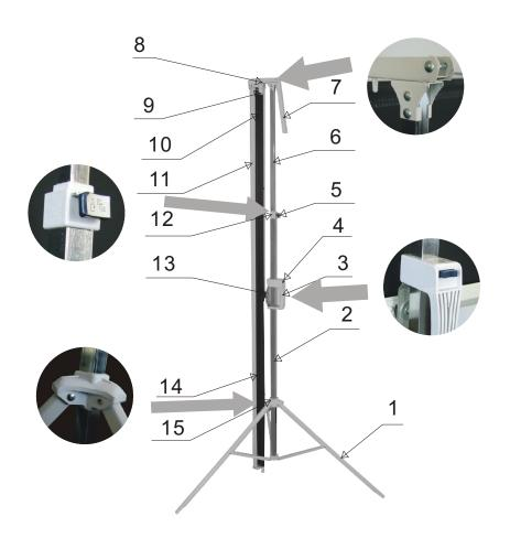
1: tripod 2: adjust tube 3: handle 4: handle button 5: adjust key 6: drop tube 7: rotary pole 8: topside tow bar 9: poling 10: screen 11: housing 12: extremity piece of square tube 13: rotary locking pieces 14: hang strip 15: tripod fork
